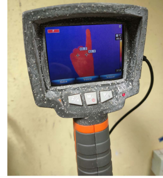
Fig. 8. Sonel KT – 384 FIR-TIC used in the data acquisition process.
