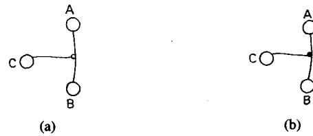
Fig. 16. (a) A stimulating modifier of the link connecting the nodes A and B, (b) A deactivating or inhibitory modifier of the link connecting the nodes A and B.
