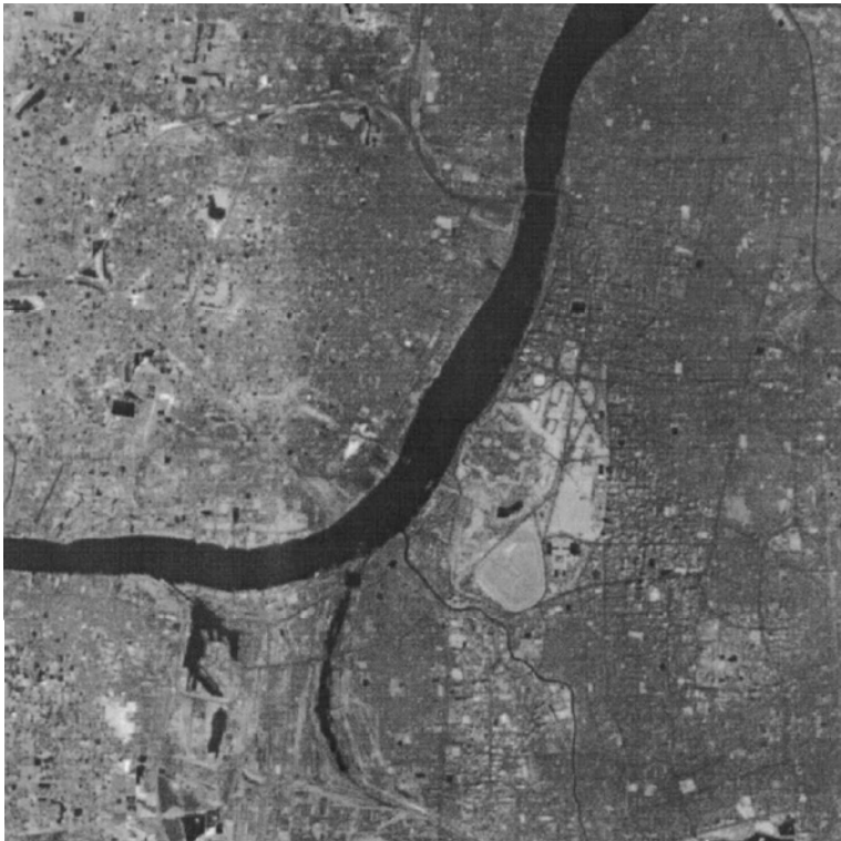
Figure 6. SPOT image of Calcutta in the near-infrared band (band 3). The image is histogram stretched.
