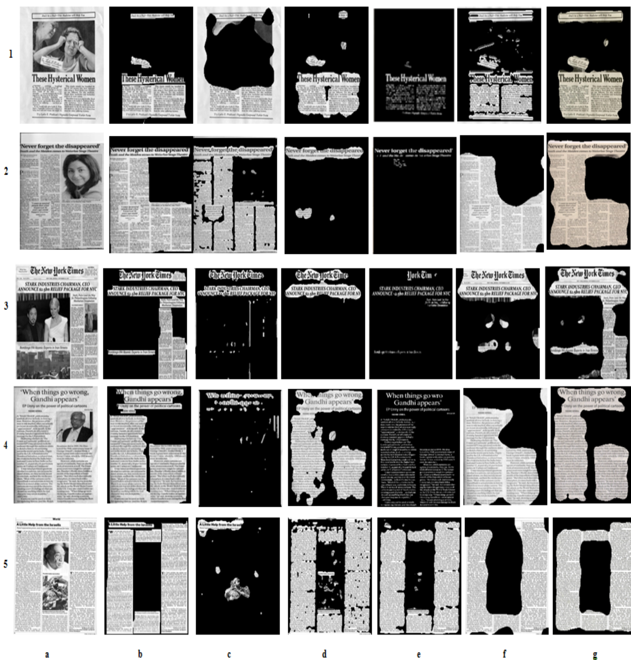
Figure 4: Column wise (a) Original test images (b) Ground truths for segmentation result (c) Results using Acharyya [25] (d) Results using Kumar [26] (e) Results using Gomez [10] (f) Results using Maji [28] (g) Results using proposed method
