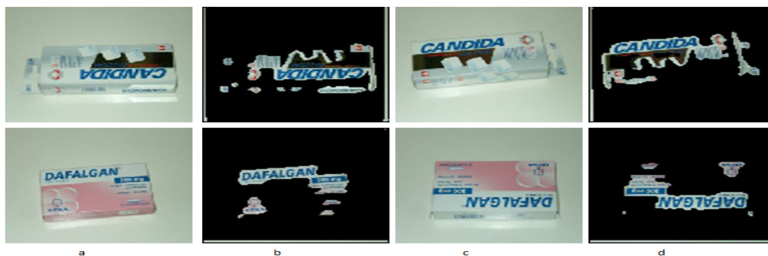
Figure 12: Column wise (a) Color text image set from Computer vision Laboratory dataset (b) Text region segmentation results of corresponding images in (a) in the same sequence, using the proposed method. (c) Another set of Color text image set corresponding to the same row in (a) with the different orientation (d) Text region segmentation results of corresponding images in (c) in the same sequence, using the proposed method.
