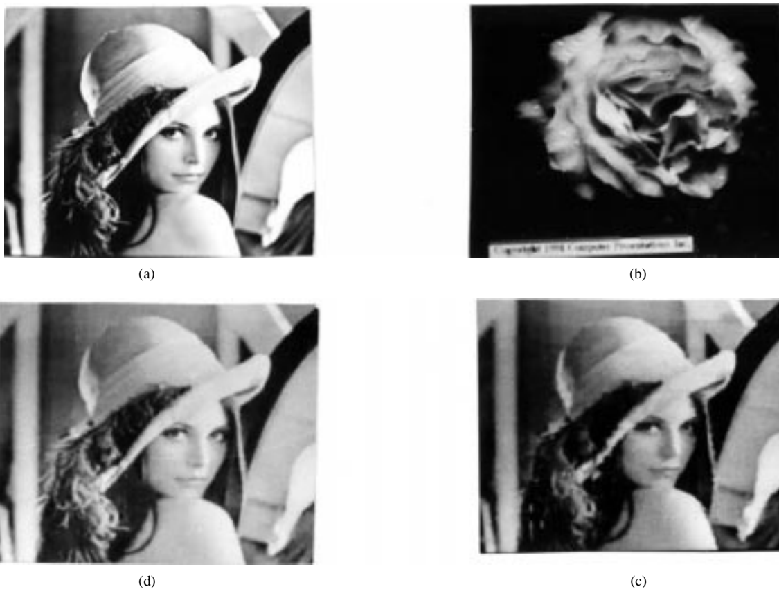
Fig. 1. (a) Original Lena image. (b) Rose image. (c) Decoded Lena image after ten iterations using single level with classification scheme with the starting image as Fig. 1(b). (d) Decoded Lena image after ten iterations using two level with classification scheme with the starting image as Fig. 1(b).
