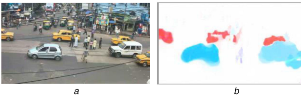
Fig. 3 Annotation of occluded objects in motion using optical flow [19]
