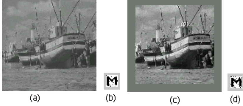
Figure 4.8: (a) Watermarked image after sharpening operation; (b) Extracted watermark ; (c) Watermarked image after cropping operation; (d) Extracted watermark
