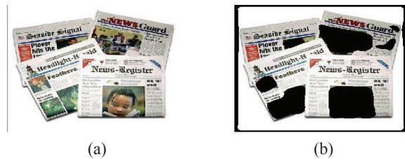
fig 4.(a) image of different newspaper at different angles.(b) segmented out text portion.
