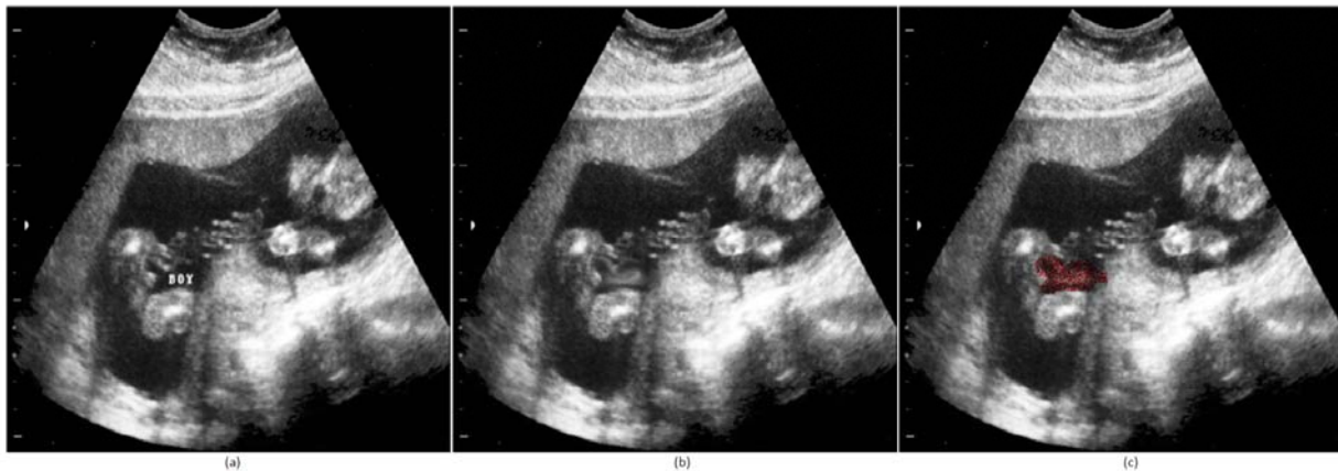
Fig. 11 – Tamper localization (a) original watermarked image, (b) tampered watermarked image, (c) tampered region. (For interpretation of the references to color in text, the reader is referred to the web version of this article.)
